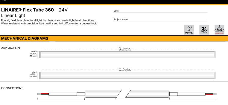
96 in. White Bare Lead 18/2 AWG UL 2464 Wire with Strain Relief
